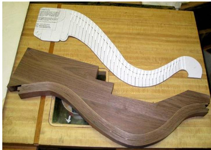
This picture shows a template for marking out the neck of a harp. The template is at the top and is made from thick card.
